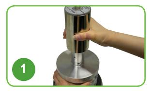
Lay Sample Processing Horn upside-down on a flat surface. Carefully attach converter by tightening clockwise with hands.
