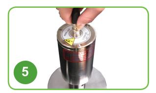
Connect one end of the *Converter Cable* to the bottom of the *Converter*. Make sure it is securely attached by turning the fastening mechanism clockwise at the end of the cable.
