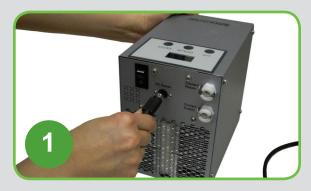
Connect the *Power Adapter's* cord to the back of the *Recirculating Chiller*.
