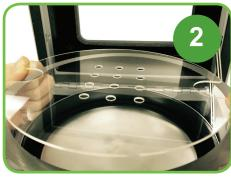
Place the *Tube Rack* into the *Sample Processing Horn* so that it rests on the gray inner rim inside the reservoir.
